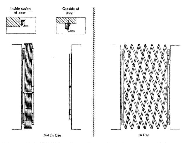
This gate can be installed inside the casing of the door or outside the door, see above. It will pivot out of the way when not in use. The gate can be mounted on the left or right. Simply turn the gate upside down to mount on the opposite side.
